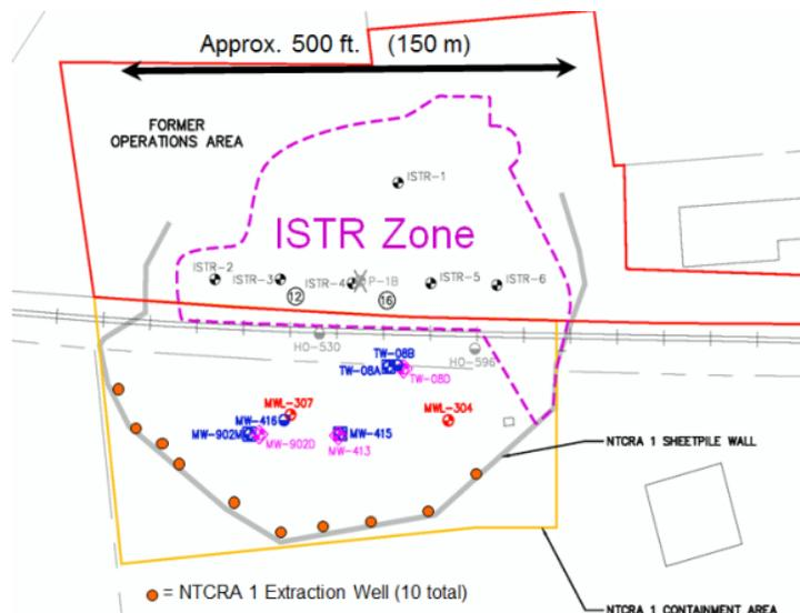
**FIGURE 3. Site layout with ISTR zone, selected monitoring wells, and NTCRA 1 overburden groundwater extraction wells.**
