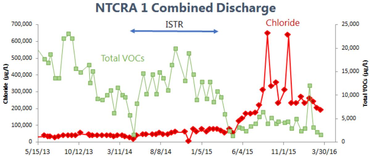
**FIGURE 8. Chloride (red) and total VOC concentrations (green) in NTCRA discharge (untreated). Blue “ISTR” arrow indicates when thermal treatment occurred.**
