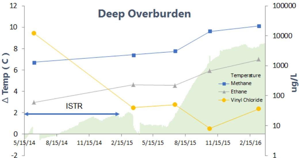
**FIGURE 6.** Temperature changes and chemical concentrations at deep overburden monitoring well MW-415. Note the decrease in vinyl chloride with the increase of methane and ethane. However, temperature and chemical data is slower than the shallow overburden. Blue “ISTR” arrow indicates when thermal treatment occurred.
