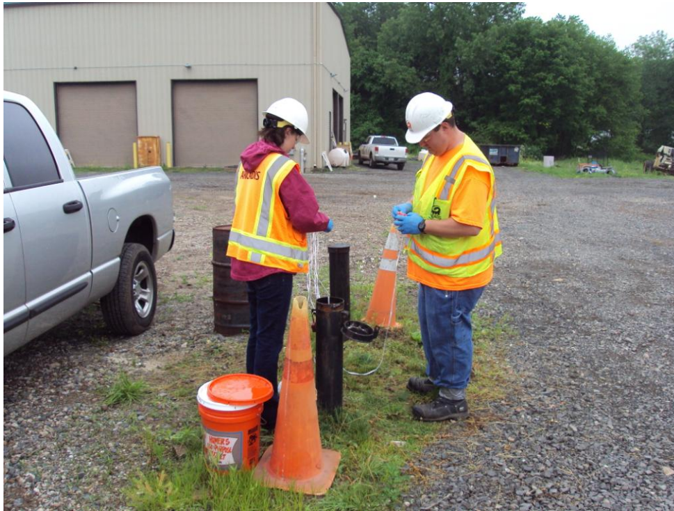
Date: 6/10/2014 Collection of groundwater sample using hydrasleeve method.
