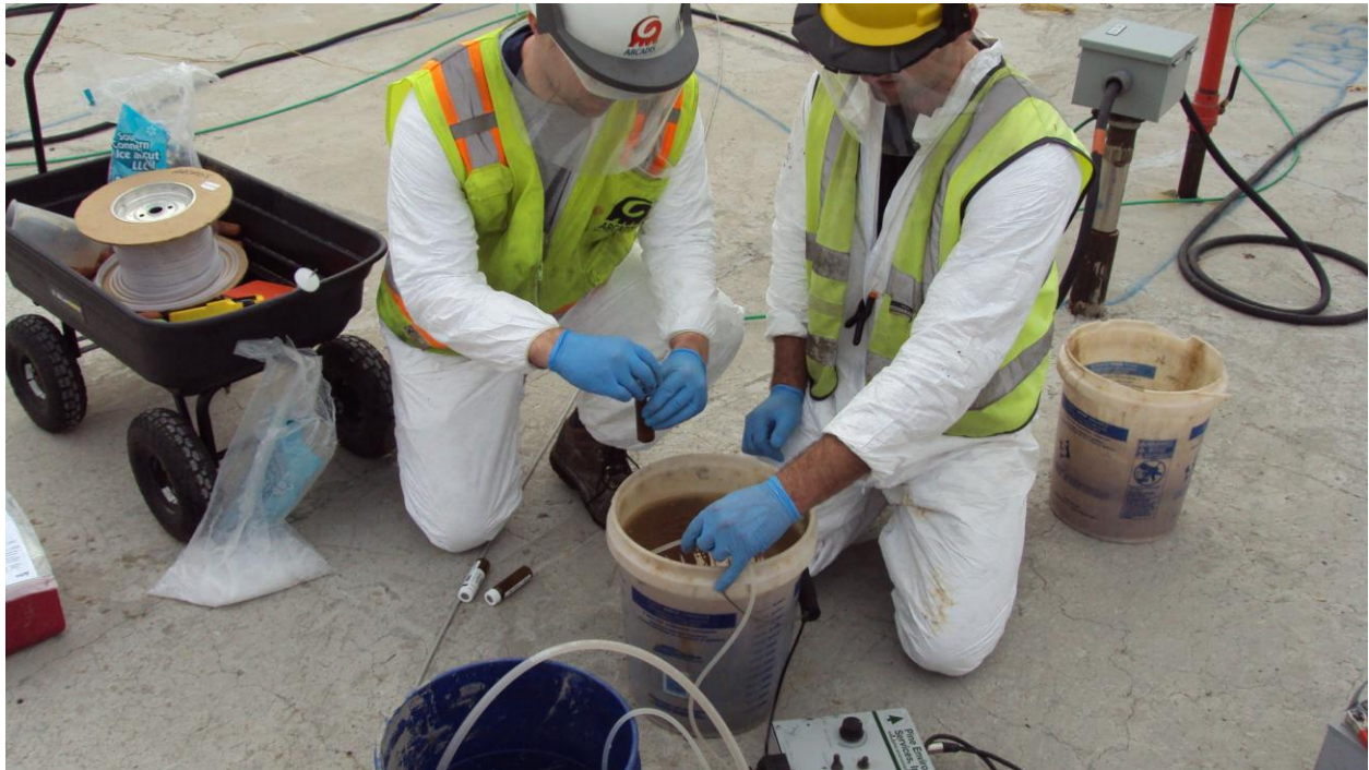
Date: 11/12/2014 ARCADIS collecting groundwater sample from ISTR-2
