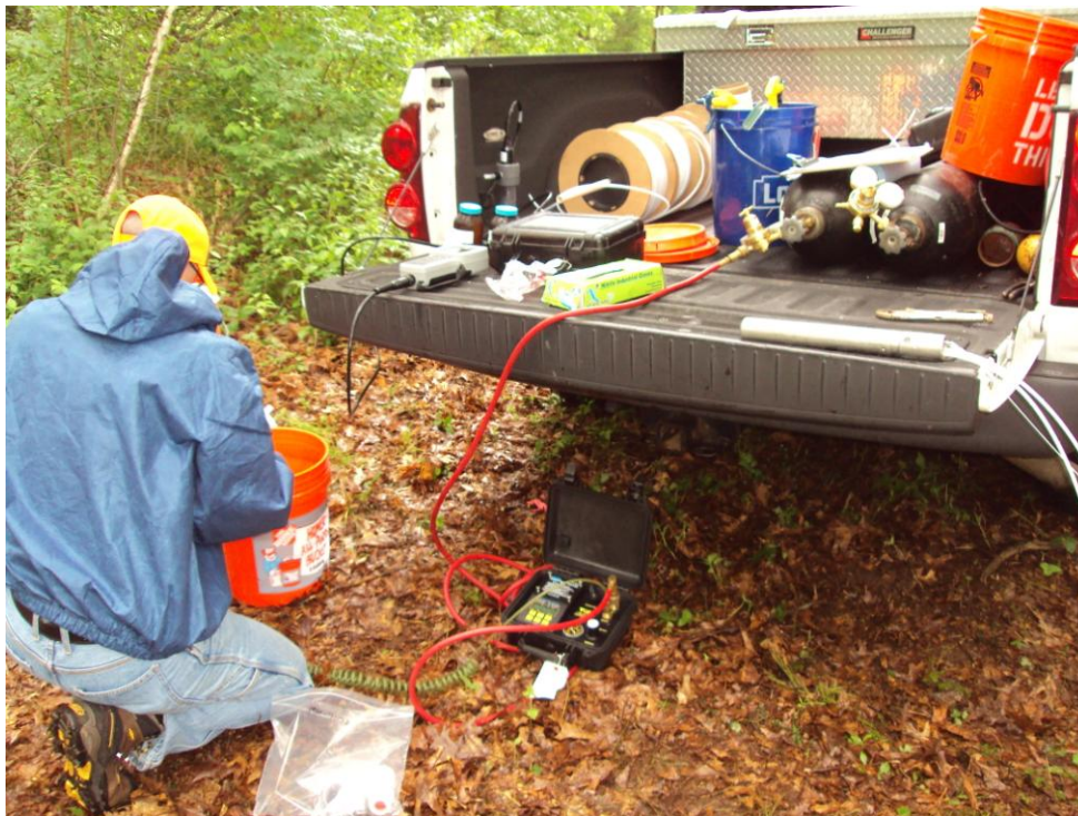
Date: 6/10/2014 Collection of groundwater sample using low flow sampling method.
