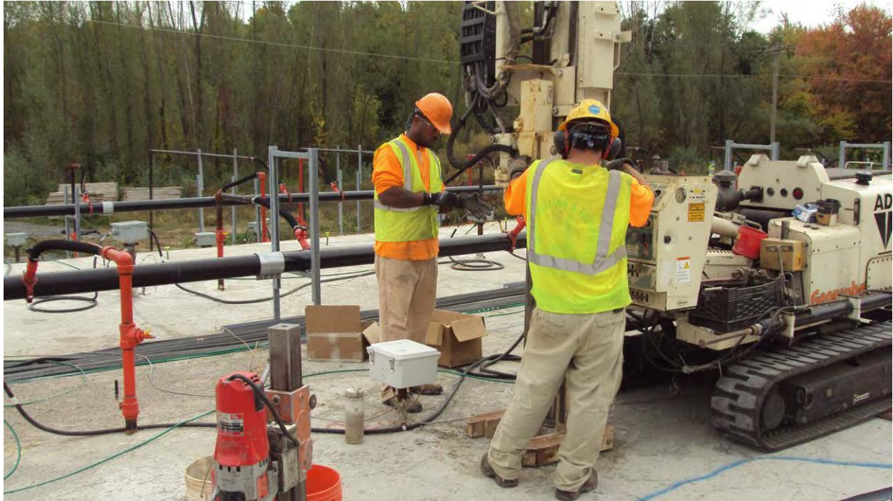
Date: 10/14/2014 Process of drilling to collect a Phase I interim soil sample.
