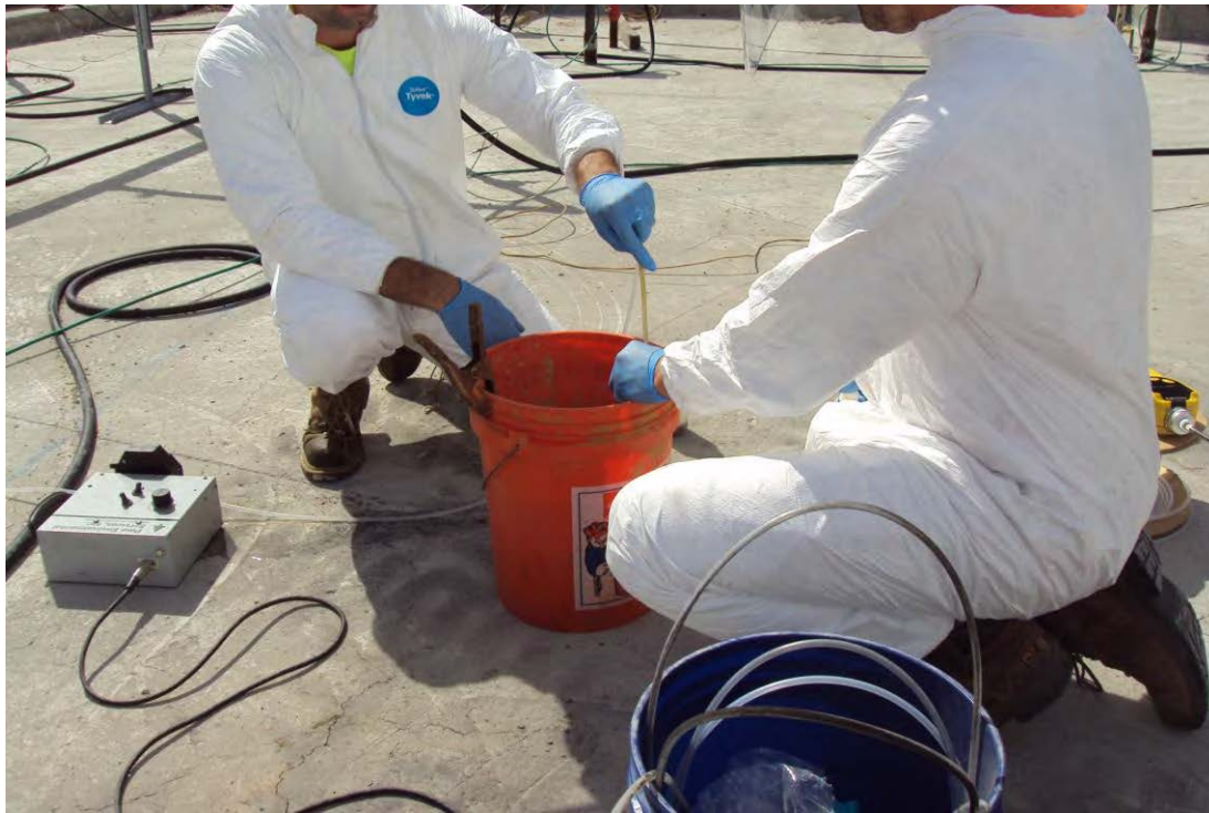
Date: 9/3/2014 Sampling ISTR groundwater monitoring well ISTR-4
