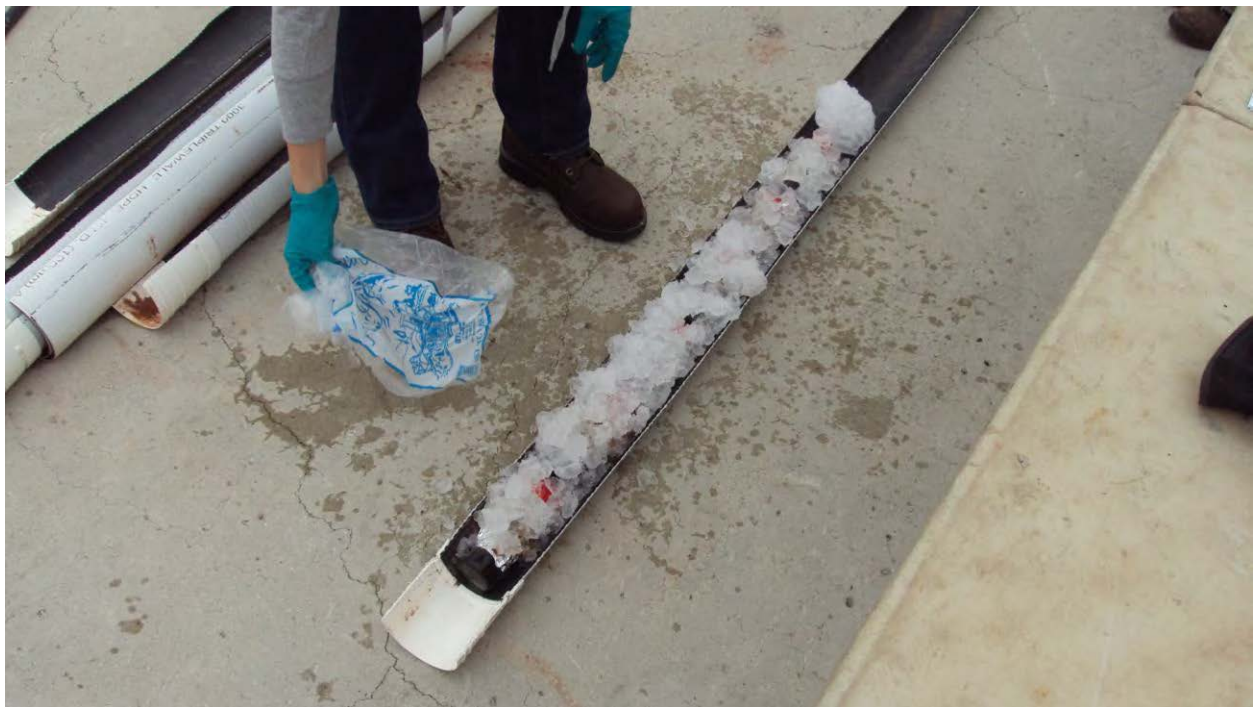
Date: 10/13/14 Typical example of cooling hot soil sample (collected during Phase I interim sampling).
