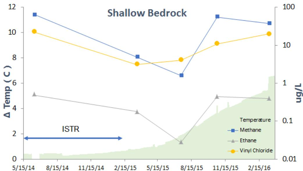
**FIGURE 7. Temperature changes and chemical concentrations at shallow bedrock monitoring well MW-416. The lack of consistent concentration changes and the slower temperature change are attributed to the fact that this well is within the bedrock, which is approximately one order of magnitude less permeable than the overburden. Blue “ISTR” arrow indicates when thermal treatment occurred.**
