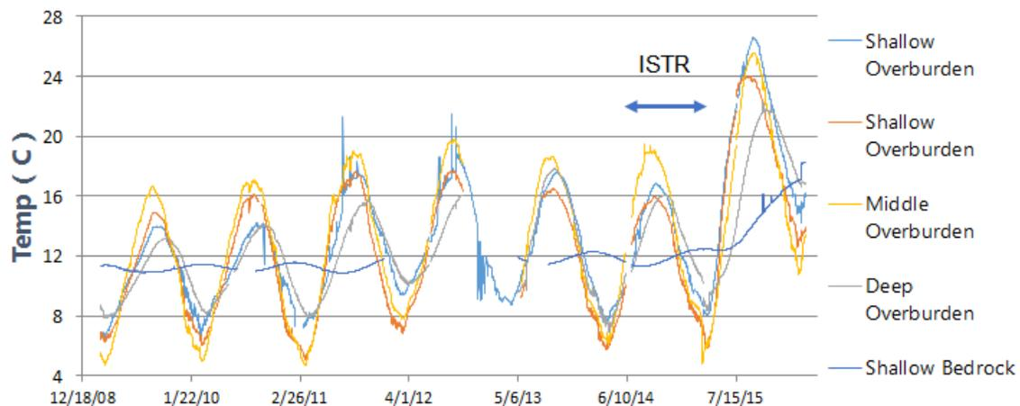
**FIGURE 4. Temperature fluctuations at monitoring wells approximately 25 meters downgradient of thermal treatment zone. Blue “ISTR” arrow indicates when thermal treatment occurred.**
