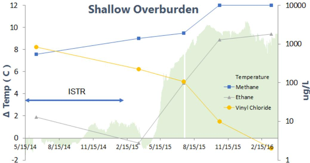
**FIGURE 5.** Temperature changes and chemical concentrations at shallow overburden monitoring well MWL-307. Note the simultaneous decrease in vinyl chloride with the increase of methane and ethane. Blue “ISTR” arrow indicates when thermal treatment occurred.
