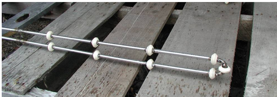
Figure 4.2. Proprietary TerraTherm Heater Element used inside each Thermal Conduction Heater Boring. The metal rod has a diameter of approximately 0.5 inch (1.2 cm). The white beads are ceramic isolators. Electric power flows through the steel rod, causing it to heat resistively. The design is covered by one or more of the following: U.S. Patent Nos. 5,190,405, 5,318,116, 6,485,232 and 6,632,047.
